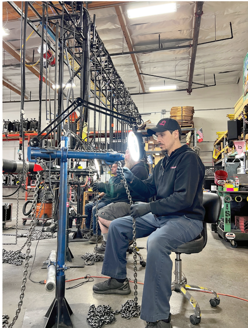
Ron Guardado, Kish Rigging’s ETCP Certified Motor Department Head, inspects a chain for a CM Chain Motor hoist.
