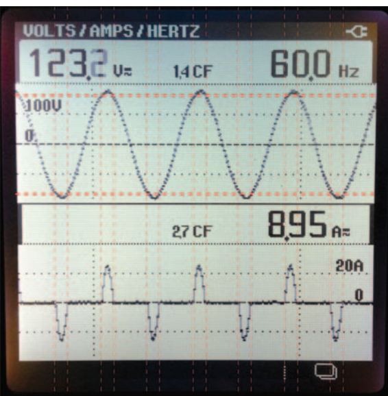
Figure 3 – When the applied voltage exceeds the charge on the capacitors, current flows, which is why current is drawn in pulses.
