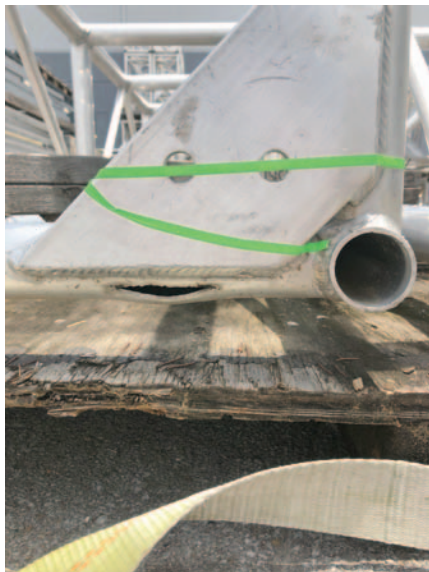
Figure 3 – Ruptured tube in truss end ring is typical of damage caused when water enters a tube and is then exposed to freezing temperatures. This can happen on jobsites or while the equipment is being transported or stored.
