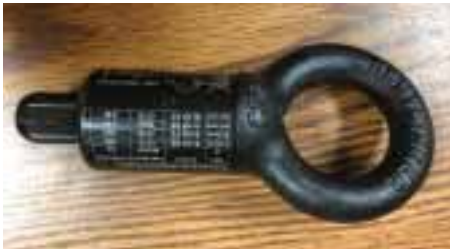
This type of device was used inappropriately, in conjunction with the wire rope, as a rigging point to suspend the LED wall in the May 2019 accident in Las Vegas.
