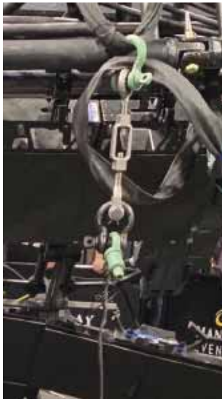
The adjustable device used in the LED wall accident in Las Vegas, similar to the one in this picture, cut through the wire rope that had been inserted through the device.
