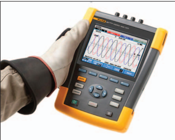
A power quality meter can be used to capture voltage transients, sags and swells, and other power disturbances.
