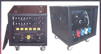
A LEX Rack<sup>TM</sup> featuring (2) 6 x 2500 Watt Lex Electrol Dimmers, GFCI protection module, and PD80 3  $\varnothing$  to single  $\varnothing$  external power distribution.
