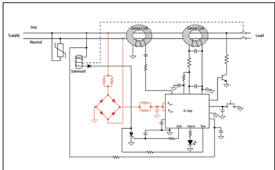
A schematic diagram of a GFCI shows the components, including an integrated circuit chip, which requires a supply voltage to operate (shown in red). If the GFCI is connected to the output of a dimmer, the supply voltage can be dimmed to the point that it drops low enough that the IC chip stops working. If the dimmer is connected to the output of the GFCI, the supply voltage for the GFCI is maintained throughout the dimming curve.
